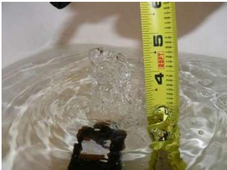
If the filter, spout and tubes are all fine, then please follow the instructions for cleaning your pump "from the inside out". Once you have cleaned the pump like this, try it in your sink with 3 inches of water; the water spray should extend about 1.5 inches over the surface of the water with a 6 volt power supply, or 1 inch with a 4.5 volt power supply.
